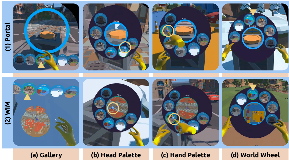
Figure 1: Eight virtual world switching interfaces that support fast and seamless transitions across different virtual environments. Two preview types are used: (1) Portal and (2) World-in-Miniature (WiM). Four interaction metaphors were derived: (a) Gallery, (b) Head Palette, (c) Hand Palette, and (d) World Wheel. The selected environment is indicated by a yellow arrow ((a) and (d)) or a blue spherical cursor ((b) and (c)). The latter is highlighted with a yellow circle for clarity.
