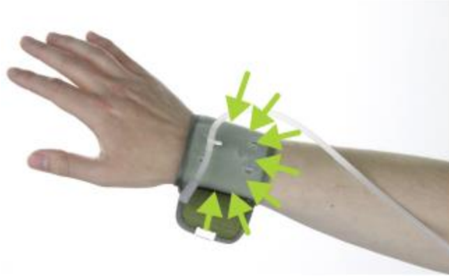
Figure 3. The compressive feedback device designed by Pohl et al. 2016 [16].
