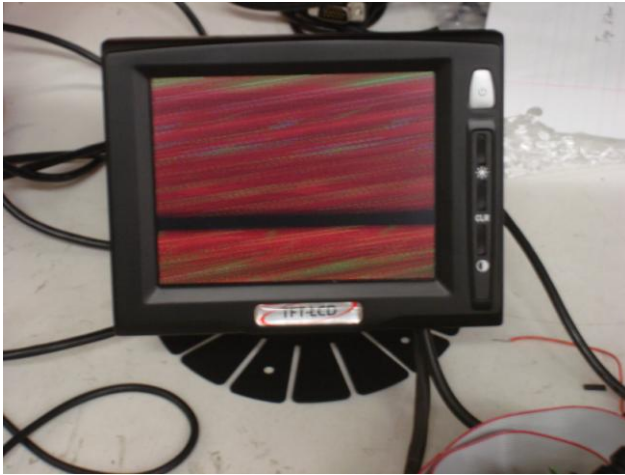
Fig. 12. Acclevision LCDP5VGA Display Unit. In this picture, it is displaying luminance values output from the camera, but without memory mapping the data.
