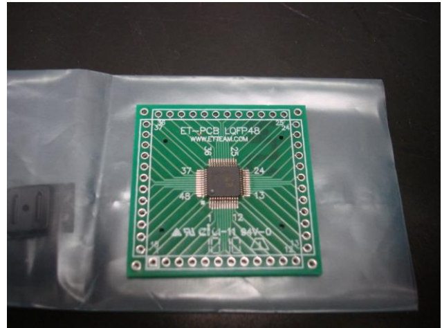
Fig. 11. DAC soldered to the breakout board
