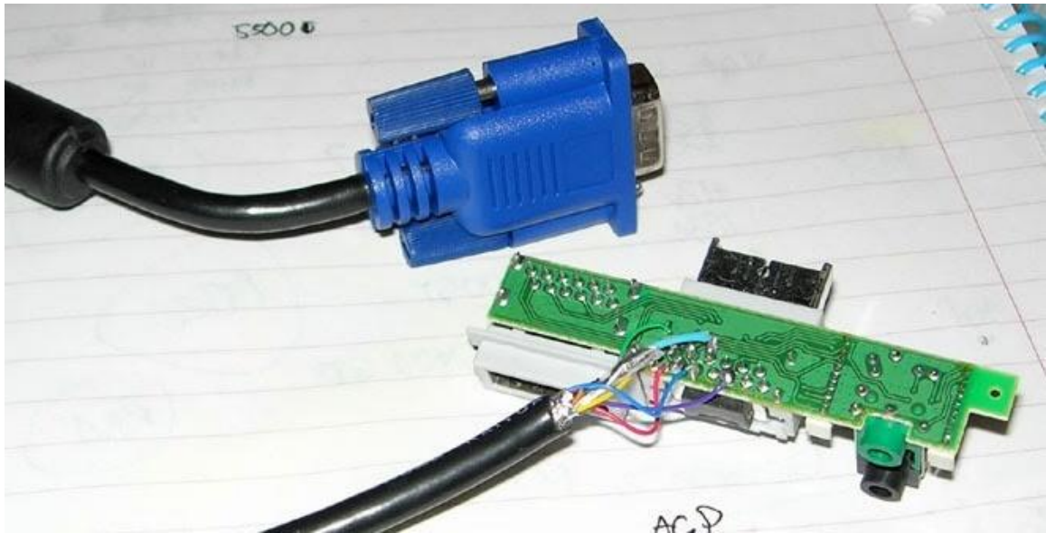
Figure 45: PSOne VGA wires soldered to the pins (Permission pending.)
