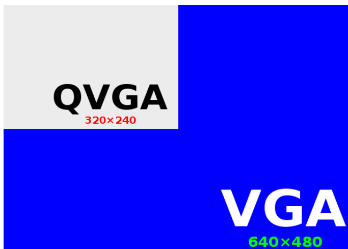
Figure 12: Comparison of VGA and QVGA resolutions
