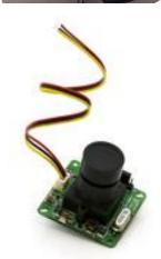
C3188A Digital Camera with OV7620 image sensor
