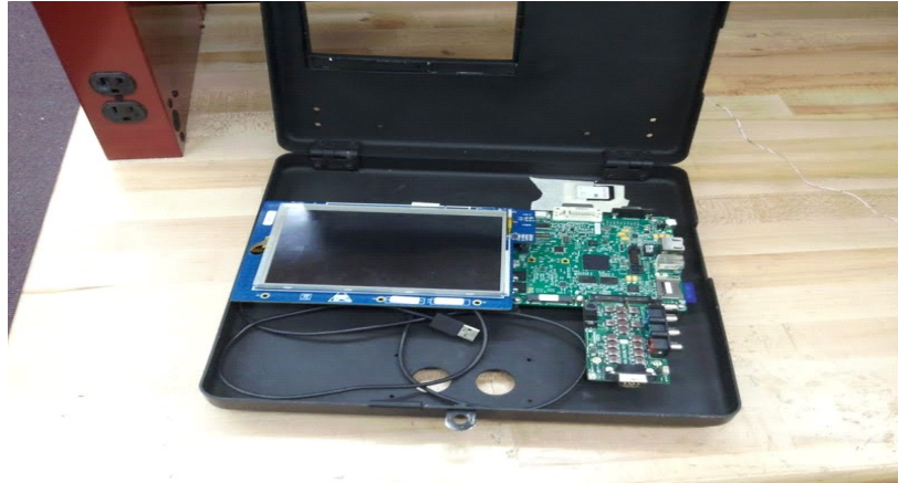
Illustration 10: I.MX51 EVK with expansion board and LCD attachments added.
