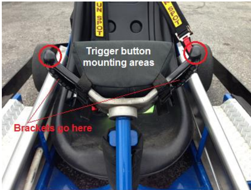
Fig.6.2.6: Trigger mounting location
