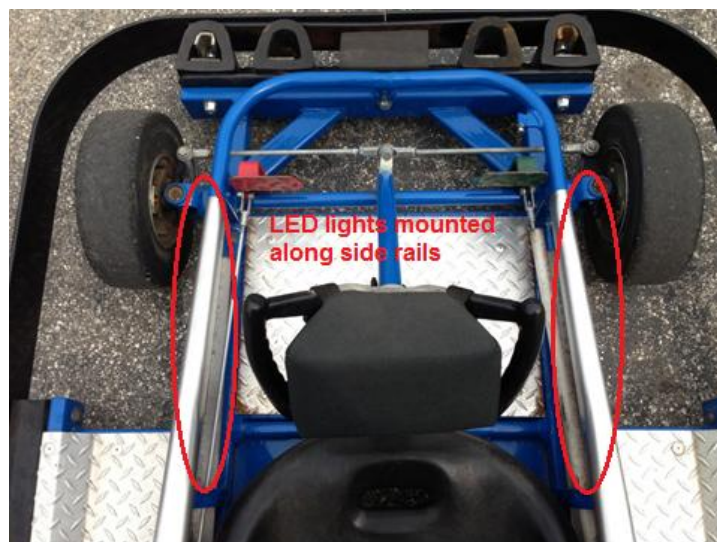
Fig.6.2.8.1: Accessory light mounting location
