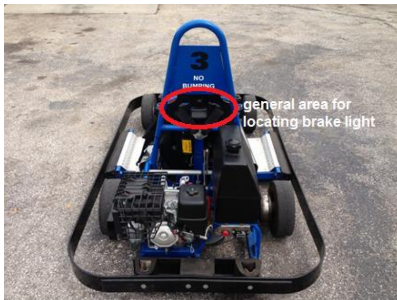
Fig.6.2.7.1: Brake Light mounting location
