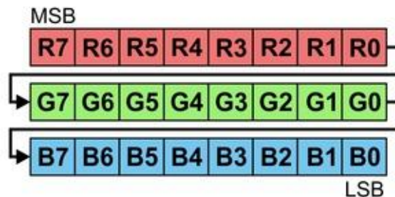
Figure 4.11.2.3 RGB 24-bit placement.
