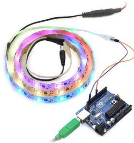
Figure 4.11.2.1 Addressable 30-RGB LED strip
