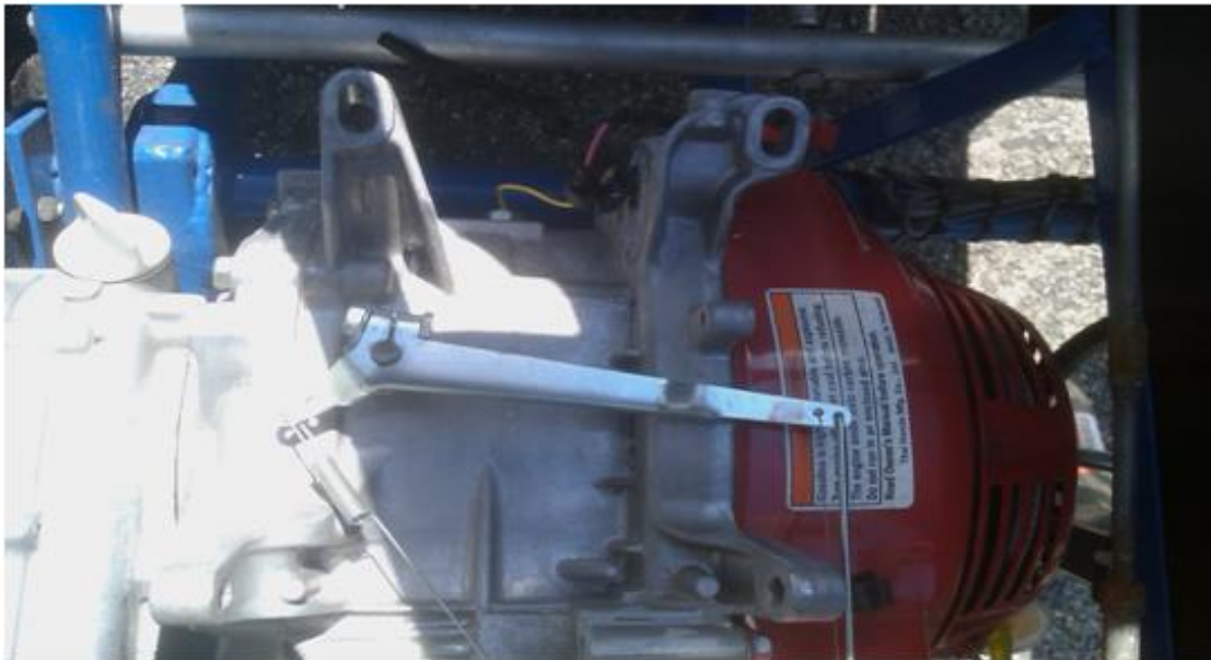
Picture 4.8.1.1: Top view of the engine governor
