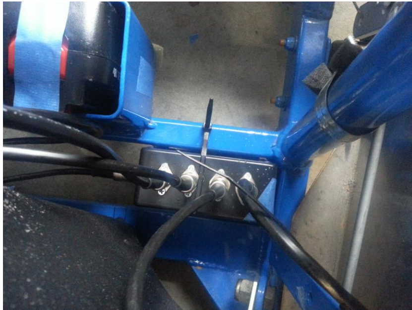
Figure 6.2.2.1: Main Module mounting location
