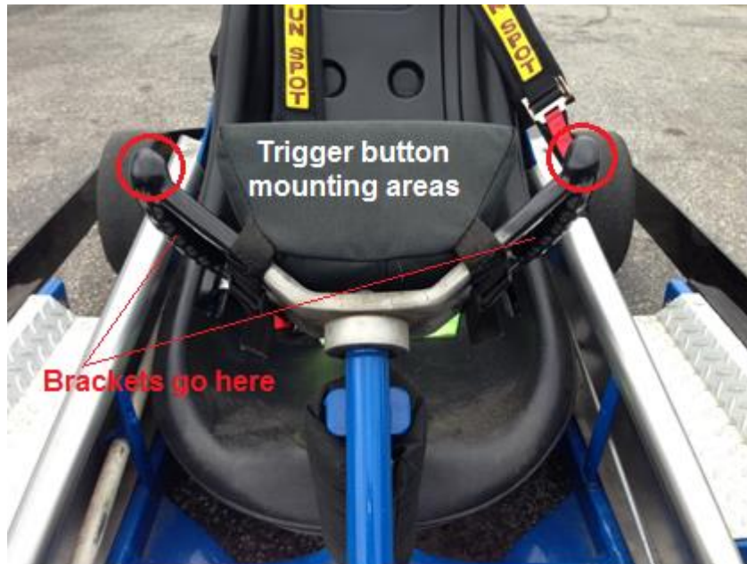
Figure 6.2.6.1: Trigger mounting location
