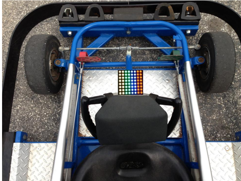
Figure 4.11.1.1: Mock-up of 8x8 LED matrix above steering wheel
