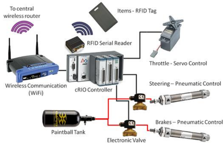
Figure 3.1.1 Waterloo Labs Mario Kart System Block Diagram Reprinted with Permission
