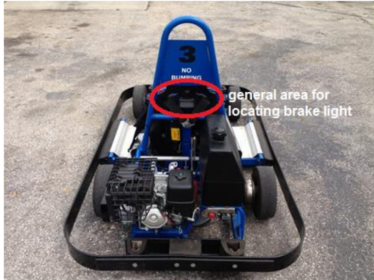
Figure 6.2.7.1: Brake Light mounting location
