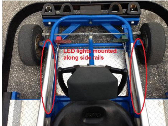
Figure.6.2.8.1: Accessory light mounting location
