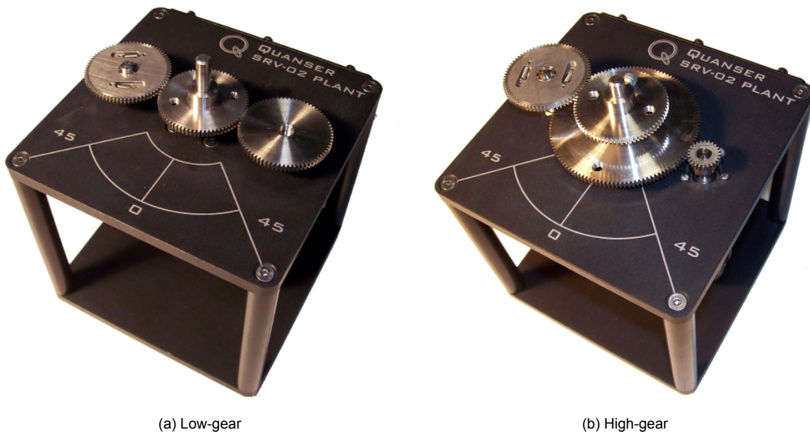
Figure 4.1: SRV02 Gear Configurations
