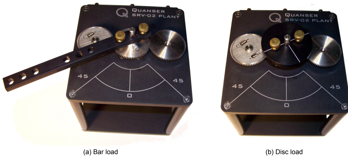
Figure 4.2: SRV02 Load Configurations
