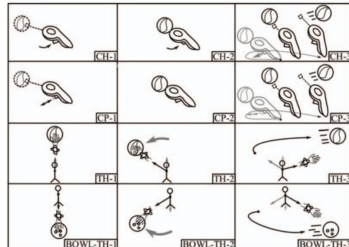
Figure 1: Throwing procedure by device configuration. **CH:** (1) hold trigger, (2) move, (3) release trigger. **CP:** (1) press trigger, (2) move, (3) press trigger. **Threshold Overarm:** (1) position near head, (2) move, (3) cross threshold. **Threshold Underarm:** (1) position near hip, (2) move, (3) cross threshold.
