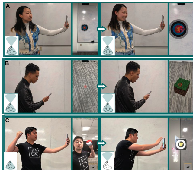
Figure 1: Cam-2-Cam combines front and rear-facing cameras to expand smartphone AR (Left), shown through three apps: A. Face TriggAR (wink), B. Mouth Craft (mouth open), C. Mirror ThrowAR (free-hand) (Right).
